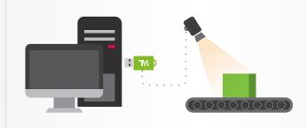
■ TM AI+<sup>TM</sup> AOI Edgecan be installed on any personal/industrial computer at production lines. After connecting the computer to external camera, the user can perform vision tasks like item recognition, image enhancement and measurement through TMvision™.
