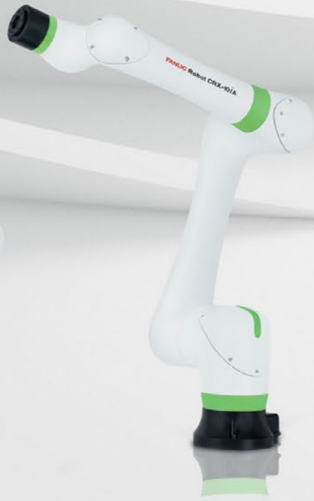
CRX-10iA Payload: 10 kg Reach: 1,249 mm
