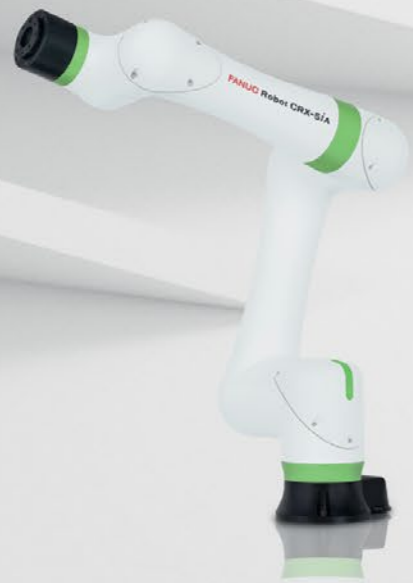
CRX-5iA Payload: 5 kg Reach: 994 mm
