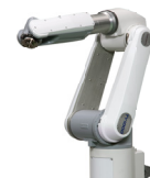
TV1000 Payload: Up to 5 kg Arm Length: 1000 mm
