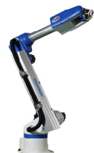
TVM1500 Payload: Up to 10 kg Arm Length: 1500 mm
