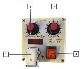
So as to comply with the **EMC** standard, the circuit is equipped with filters with leakage currents to earth lower than 1mA. The circuit supplies the vibrator with a pulse width modulated control signal (**PWM**) adjustable both in **Amplitude** and **Frequency**. This signal is compensated with regards to line voltage variations.
