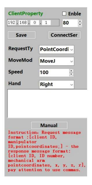
For coordinates, select the appropriate motion mode, speed, and hand system to execute the transmitted coordinates. Message format is as follows:
